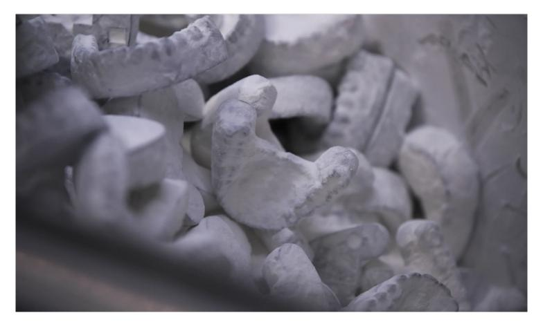
After being printed, each arch must be cleaned by hand before the molds are used to create liners for each customer.
